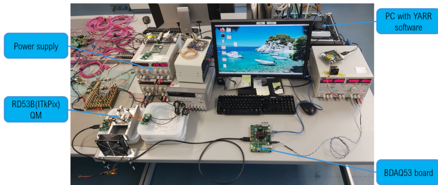
Figure 6.13.: The lab setup used to develop the YARR software for reading out the RD53B QM using the Bdaq53 board.
