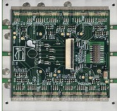
Figure 5.5.: The Quad module used in the ITk pixel detector [72].
