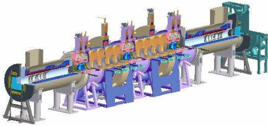
Fig. 3. Drawing of the MICE experiment [51]. The beam enters the experiment from the bottom left-hand corner. The beam first passes through one of the scintillator hodoscopes that form the time-of-flight system. After passing through the upstream spectrometer, the beam passes through three absorber/focus-coil modules and two cavity/coupling-coil modules before it passes through the downstream spectrometer and, a second time-of-flight hodoscope, the downstream Cherenkov counter and is stopped in the electromagnetic calorimeter. The beamline and upstream instrumentation is not shown.
