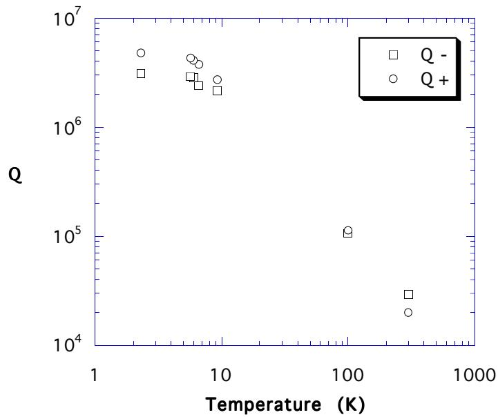
Figure 1: mechanical quality factors of mode - , 913Hz, and mode +, 931Hz, as a function of temperature.
