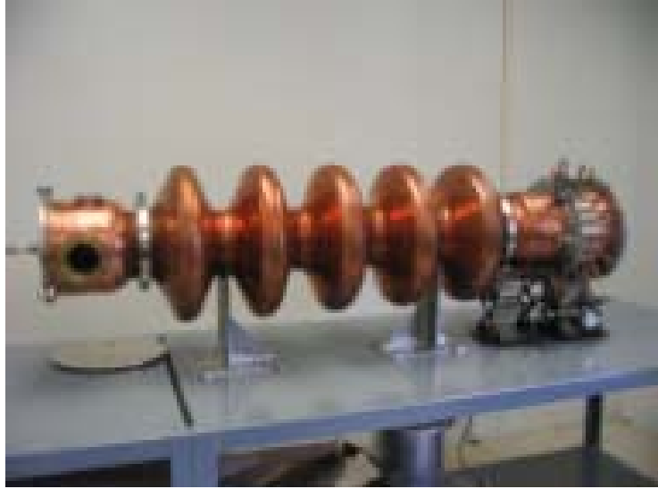
Figure 3.3: The five-cell copper cavity with prototype ferrite HOM absorber.
