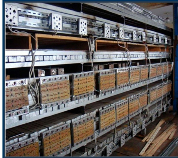
Figure 6. Hadron block of the ionization-neutron calorimeter.
