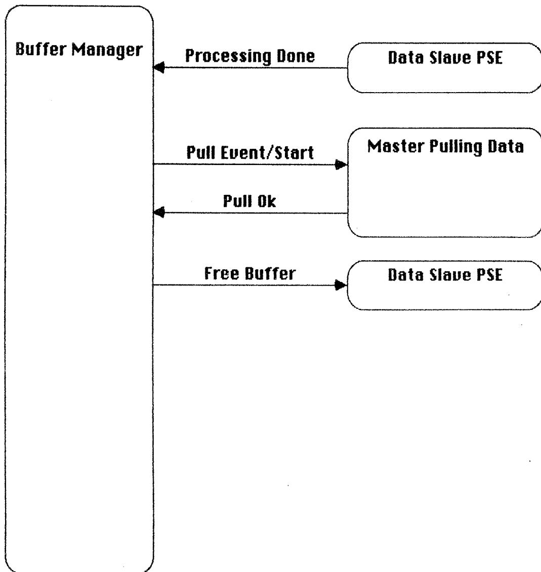
designers of the PSE hardware, it is better to base the Buffer Manager's actions on the role of a PSE in a given transaction rather than on the details of the PSE itself. For this reason, the Buffer Manager deals with the concept of a pipeline link, containing information about the roles of the participating PSEs as well as the PSEs themselves. By dealing with roles, the main loop of the pseudo-code can treat the two cases of Figures 2 & 3 identically.
