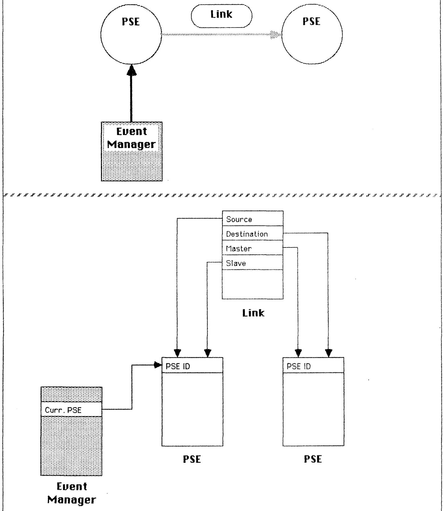
stage to a pipeline. The Event Manager is the active portion of the system. It actually executes the code of Listing 1. It keeps in its own local storage a pointer to the Current PSE, that is, the stage where the event data reside at the start of the transaction. A single pass through the code will move the data across the link and point the Event Manager to the new data location.
