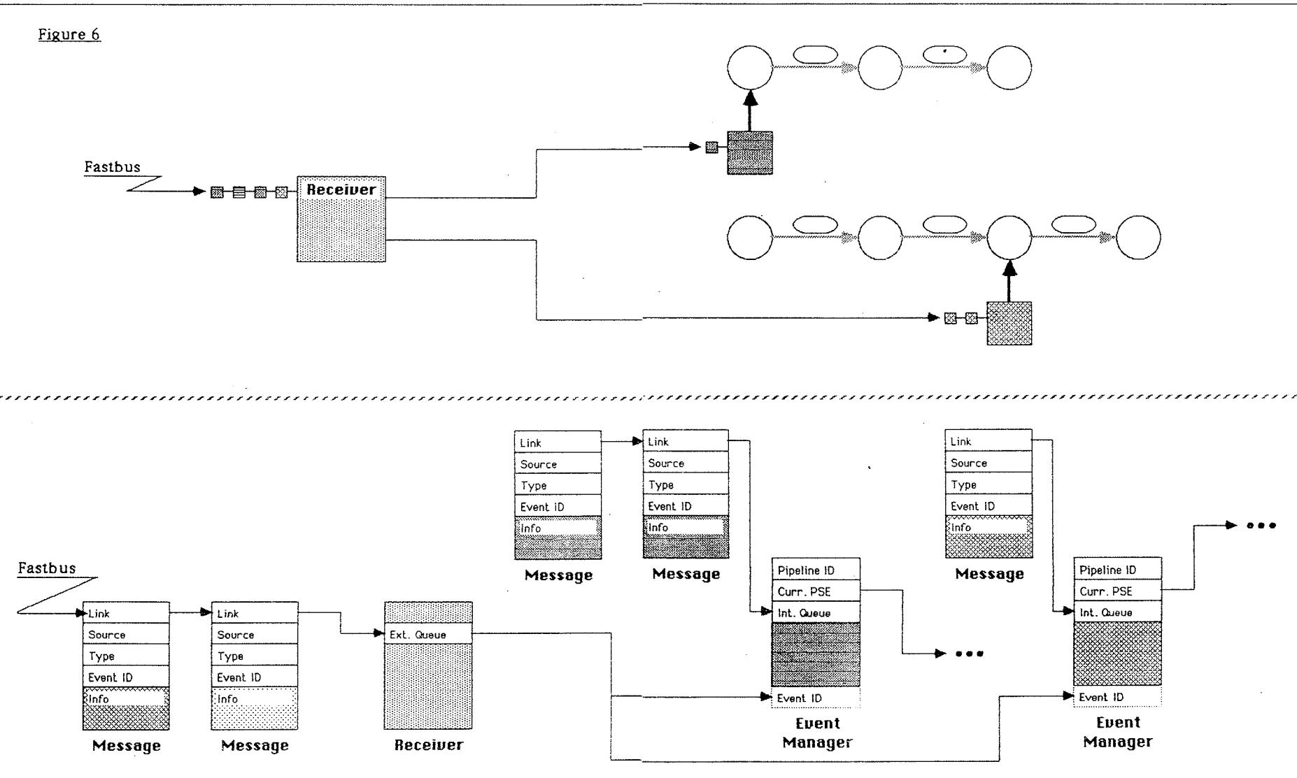
contains a Link field which points to the next item in its queue. The Link field is added to the message after its reception; it does not exist on the Fastbus.
