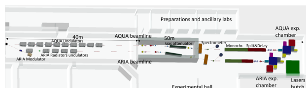
Figure 6. EuPRAXIA@SPARC LAB FEL beamlines, AQUA and ARIA layout.
