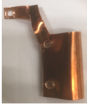
Figure 4.4 – Copper bracket encapsulating the charcoal sample.
