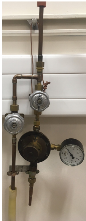
Figure 4.5 – Pressure valve used to stabilise the ^4\text{He} flux.
