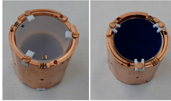
Figure 5.9 – A detector module with a top ( left ) and a bottom ( bottom ) view. On the bottom, the Ge NTD is placed [98].
