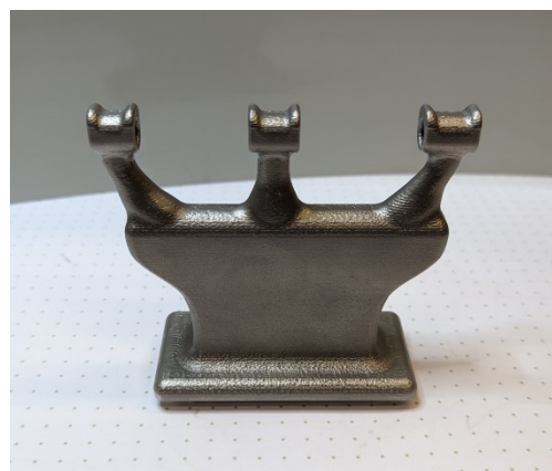
Figure 5: New geometry printed in 1.4404 stainless steel. Bottom surface and beam aperture have been CNC machined.
