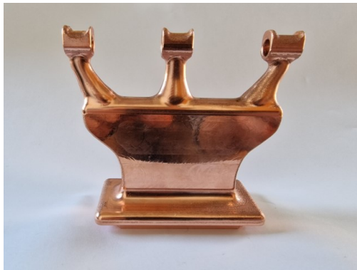
Figure 7: New geometry printed from pure copper after CNC post-processing.
