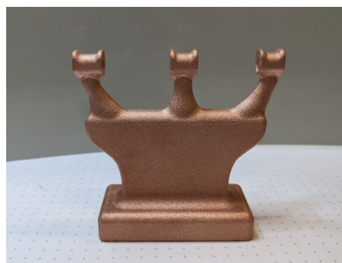
Figure 6: New geometry printed from pure copper before CNC post-processing.
