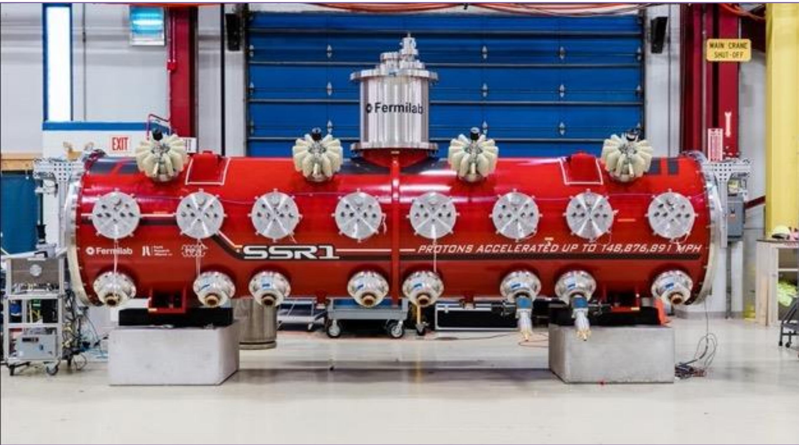
Prototype SSR1 cryomodule built for PIP-II. Implements current cutting edge SRF technology to accelerate proton beam in 800 MeV Linac.
