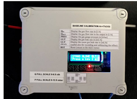
Figure 3. A photo of the front view of the SA-GLT prototype showing the LCD screen and the associated keypad.
