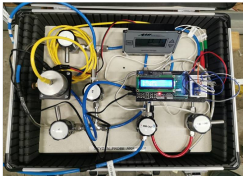
Figure 12. Photo of the “briefcase” setup (OPA-3) for monitoring the percent oxygen of a Double Wedge in Cosmic Ray Stand in BB5 at CERN.
