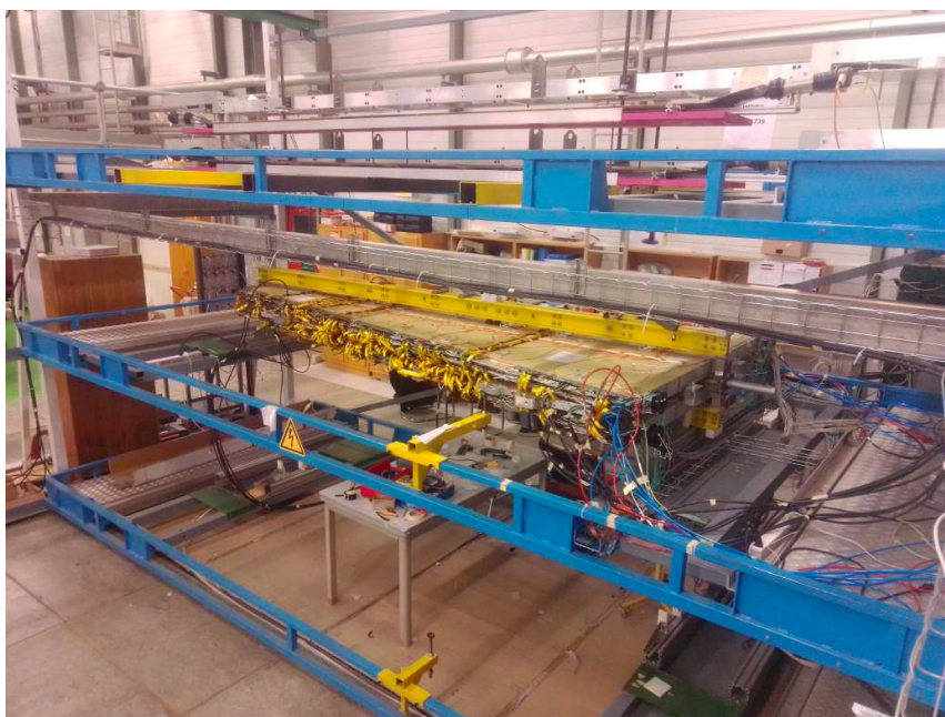
Figure 10.6.: Picture of the Micromegas double wedge cosmic ray test stand, kindly provided by [90].
