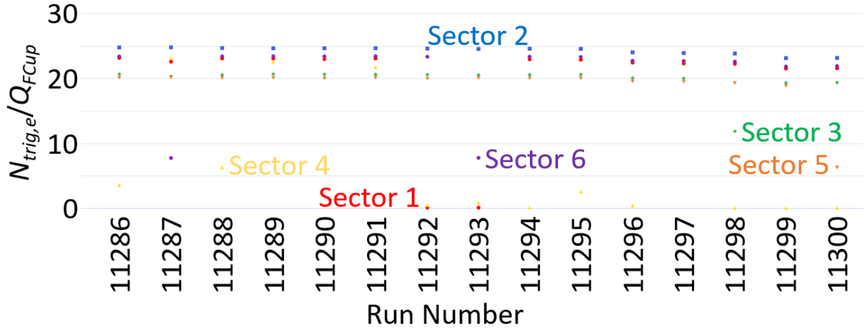
FIG. 23. The number of trigger electrons over the faraday cup charge for each of the runs considered for this analysis. Note the many runs with DAQ problems, especially with sector 4.
