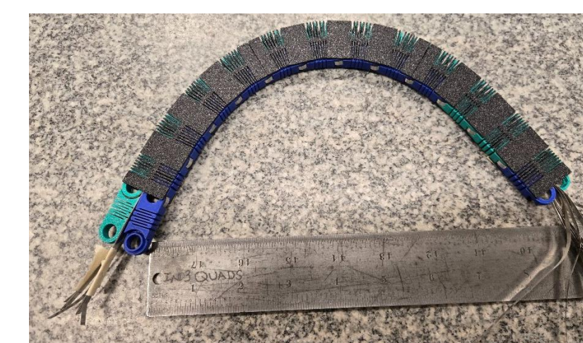
Figure 9: Arrangement of REBCO in Rutherford-like Cable
