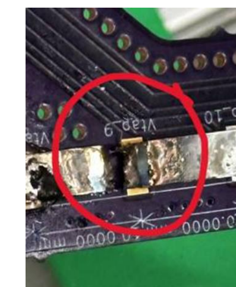
Figure 6: Resultant burn on sample
