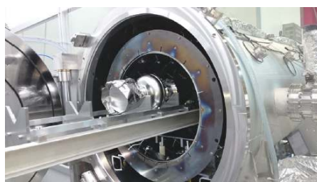
Fig. 6 N-doping of 1.3 GHz cavity
