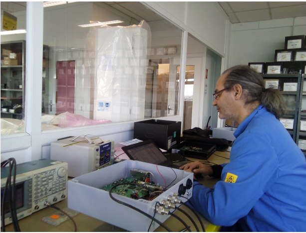
Figure 6.12: Left: David Martin testing one of the 35 Front-End unit produced at STAE in November 2017. Right: average signal levels measured at the outputs of the unit b07 for a sine wave of fixed amplitude and variable frequency. A relative variation smaller than 10% was found in the range 35-95 MHz for a majority of units.
