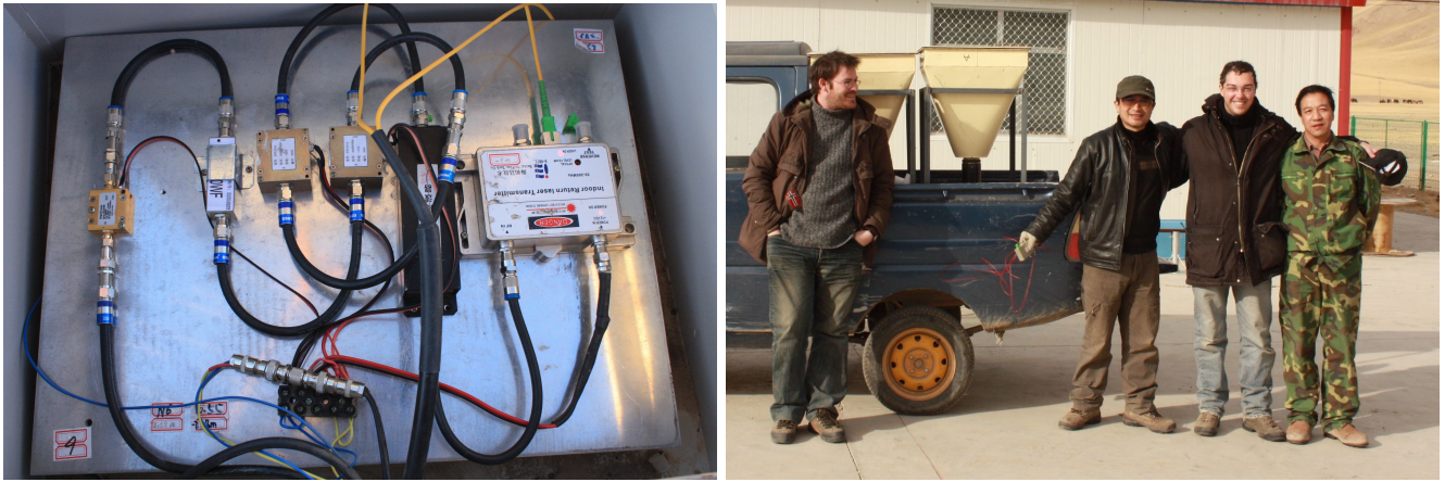
Figure 5.9: Left: a TREND15 front-end electronic board, composed of a Low Noise Amplifier (left), two 50-100MHz filters, two additional 20 dB amplification stages and an optical transmitter. The two fibers connected to the DAQ room lie atop the board. Right: TREND15 scintillators about to be deployed. Picture taken with Thomas Saugrin, Zhao Meng and Chen ShiFu, a key member of the Ulaistai staff. The scintillation plate is fixed atop a pyramidal structure which guides the light to the PMT fixed at its apex. The building in the back of the picture is the TREND DAQ room.
