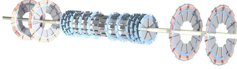
Figure 3.2: The disk/barrel design of the SMT [36].
