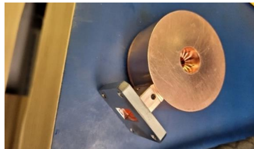
Figure 8. 10GHz, 20 vanes, coaxial magnetron used for cold test.
