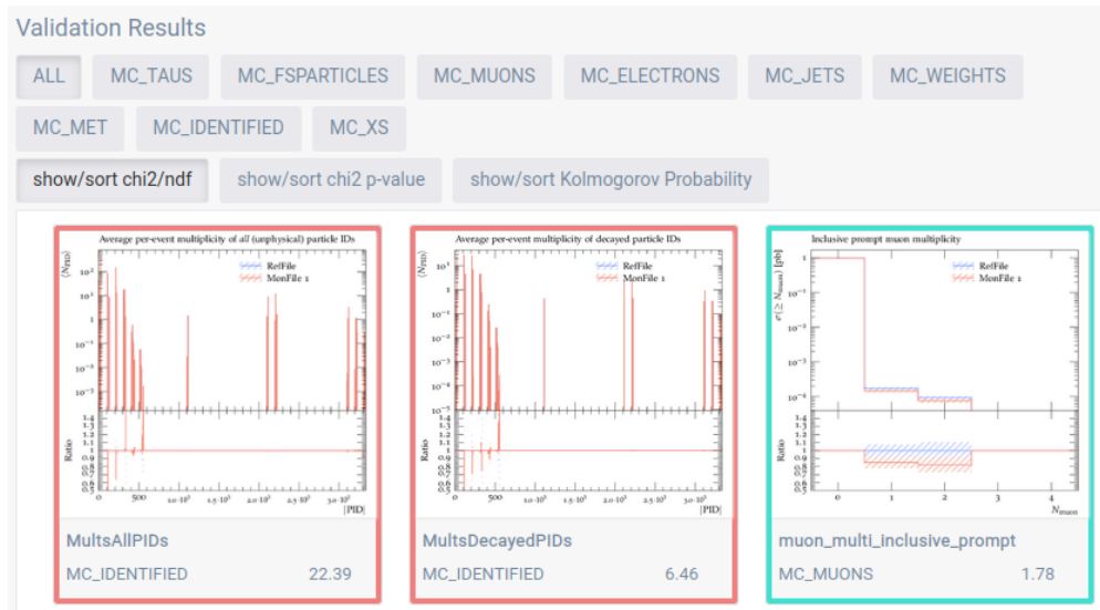
Figure A.2: Example for validation plots on the webpage. A specific analysis can be selected by the user in order to reduce the number of displayed figures. Furthermore, the test statistic used for the sorting of the validation plots can be chosen. The number in the coloured frame gives the result of the selected test statistic.
