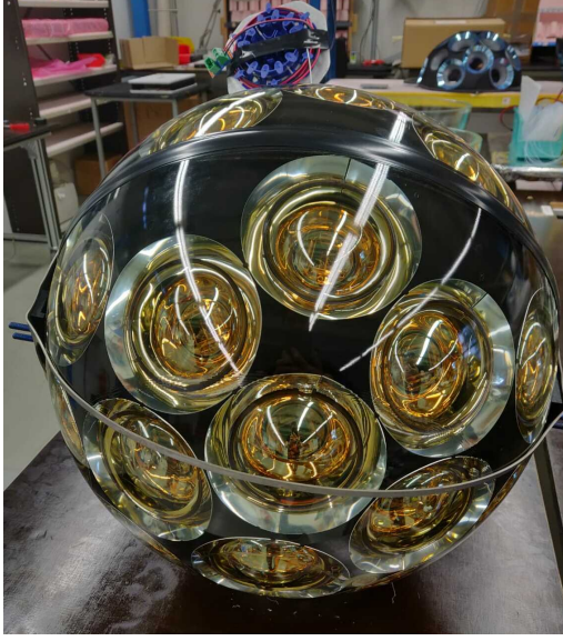
(a) A DOM, with a tilted view to see most of the PMTs from the bottom half. The golden area is the photocathode, while the silver ring around it is the reflector ring. You can see the electronic and power connectors on top.
