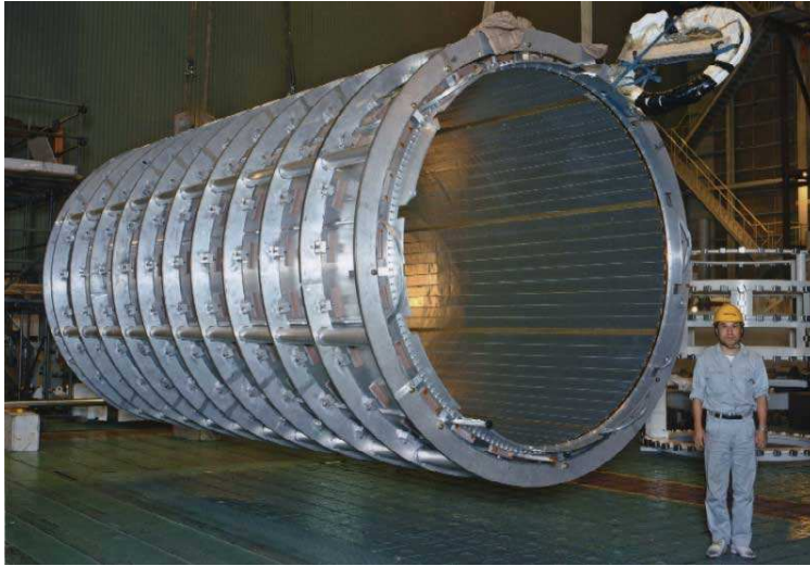
Figure 3.2: The ATLAS solenoid providing the magnet field in the ID.
