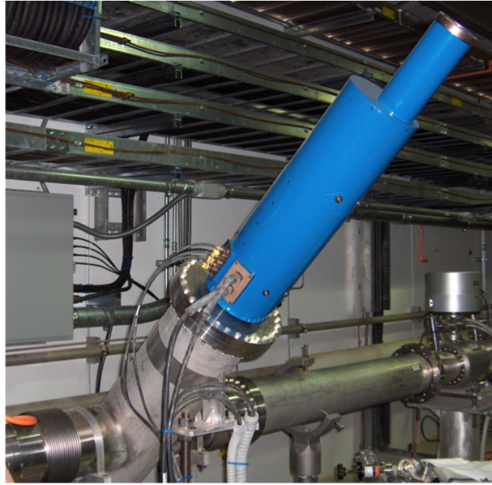
Figure A.1: Image of an RTBT Wire Scanner. Device image courtesy of S. Murray, SNS.
