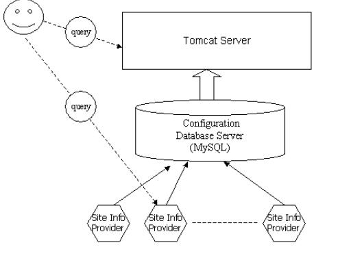
Figure 1. A prototyped architecture of the configuration monitoring system
