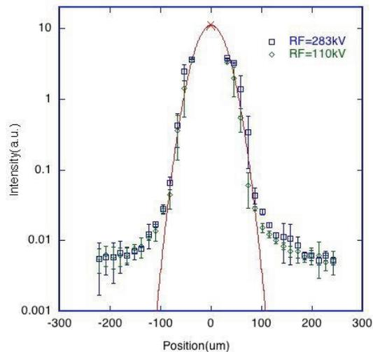
Figure 9: Distribution of the beam halo for the different rf voltage of the damping in the case of the beam intensity  $0.23 \times 10^{10}$  electrons
