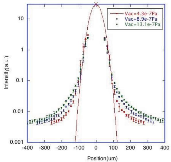
Figure 8: Distribution of the beam halo for the different vacuum condition in the case of the beam intensity  $0.45 \times 10^{10}$  electrons
