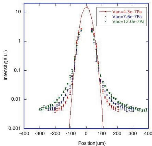
Figure 7: Distribution of the beam halo for the different vacuum condition in the case of the beam intensity  $0.23 \times 10^{10}$  electrons
