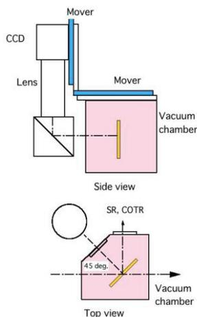
Figure 4: Layout of the YAG:Ce screen and the imaging lens
