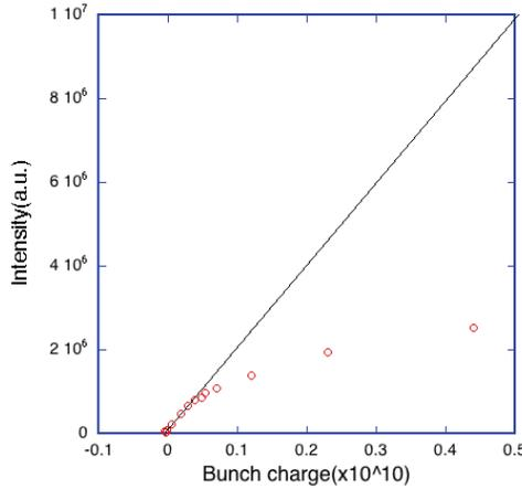
Figure 6: Light intensity of the YAG:Ce as a function of the beam charge
