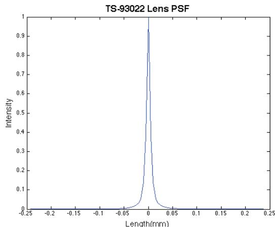
Figure 5: Point spread function (PSF) of the TS-93022 lens
