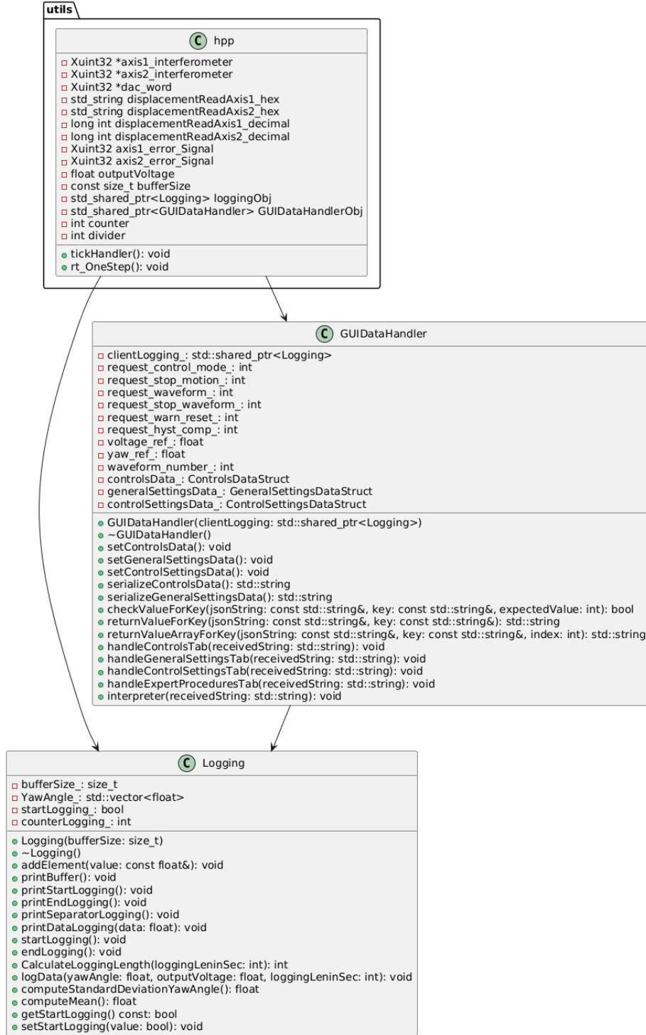
Figure 4.16: Diagram illustrating the interdependencies among the header file 'utils', Logging, and GUIDataHandler classes in the vitis application system. 'utils' integrates with both Logging and GUIDataHandler, where Logging manages logging functionalities and GUIDataHandler handles data interpretation and control modes.
