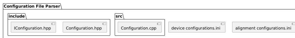
Figure 3.26: The diagram illustrates the structure of the Configuration File Parser module. It is divided into two main directories: include and src. The include directory contains header files defining class interface, while the src directory includes the source file that implements the class behavior. Additionally, the module handles configuration files essential for storing device settings and alignment parameters.
