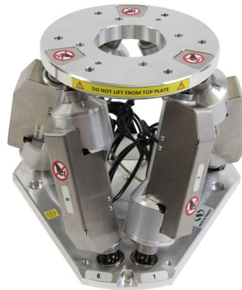
Figure 3.15: Newport HXP50-MECA with six degrees of freedom used in this work, from [26]
