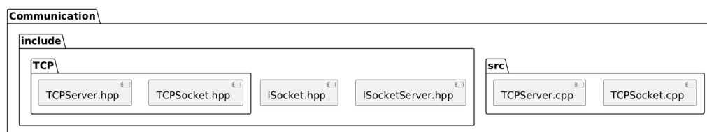
Figure 3.27: The diagram depicts the organization of the Communication module. It is divided into two main directories: include and src. The include directory contains header files for TCP communication, as well as general socket interfaces. The src directory includes the corresponding source files that implement the functionality of the TCP communication classes.
