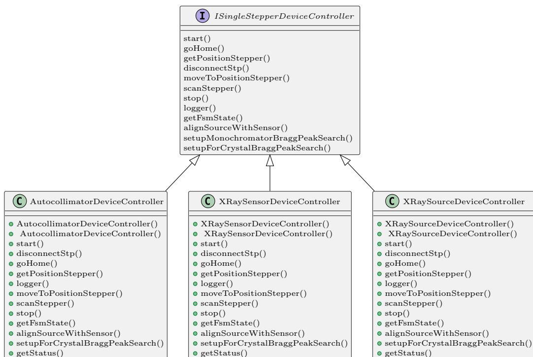
Figure 3.33: Unified Modeling Language (UML) diagram illustrating the ISingleStepperDeviceController interface and its implementations in the AutocollimatorDeviceController , XRaySensorDeviceController , and XRaySourceDeviceController classes. The interface outlines methods for controlling single-stepper devices, while each class provides specific implementations tailored for autocollimators, X-ray sensors, and X-ray sources, including alignment and scanning functionalities.
