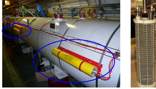
Figure 2.18: Beam Loss Monitor (BLM) in the LHC (left) and ionization chambers (right), from [19]
