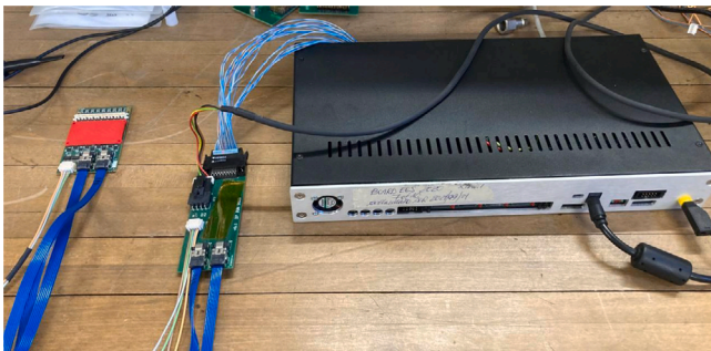
Fig. 6. New FEE readout chain in Turin laboratory, from left to right the AMBER Micromegas FEB, DLVPC board and the GEMROC module.
