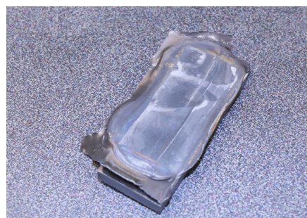
Figure 2: Sample assembly removed after the VHP process as wrapped with zirconium getter.
