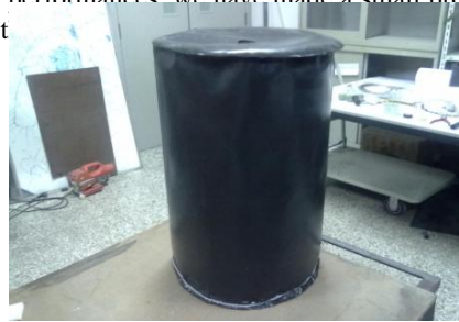
Fig.5. The liner prototype without the assembling of PMT enclosures, its diameter is 0.58 m, and height is 0.92 m.
