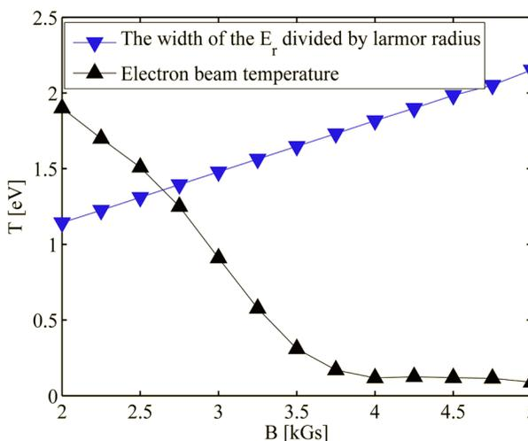
Figure 6: Dependency of the transverse temperature increase at the entrance of the toroid on the magnetic field in the gun region.
