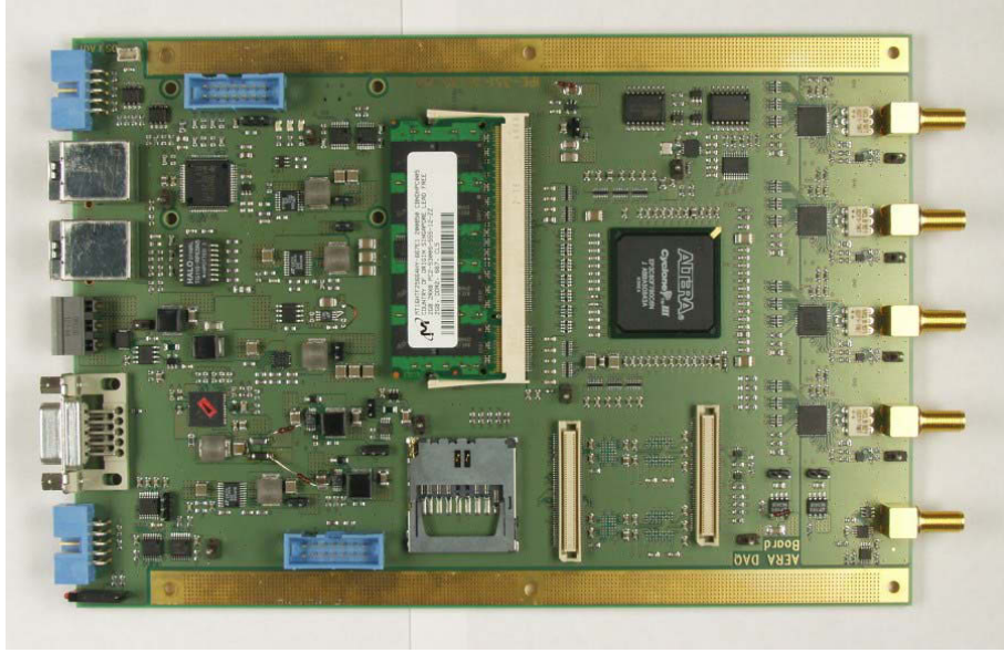
Figure 5.4.: Photograph of the AERA digitizer.
