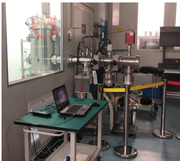
Figure 3: Magnetron sputtering device.
