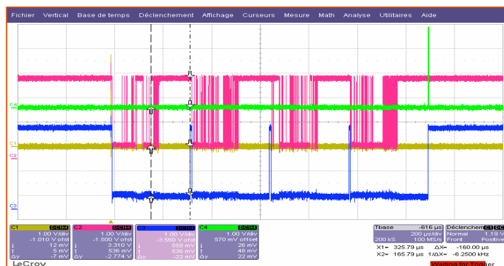
Figure 123: Four chips read-out sequentially, with the scheme described in §3.1.3. Each chip provides 128 events with 2 bits of data per event together with the BCID and chip header.
