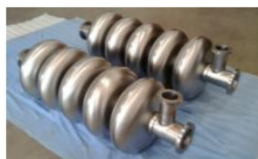
Figure 16 : S.C. elliptical cavity developed at IHEP.
