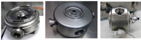
Figure 15 : S.C. Spoke cavities developed at IHEP.
