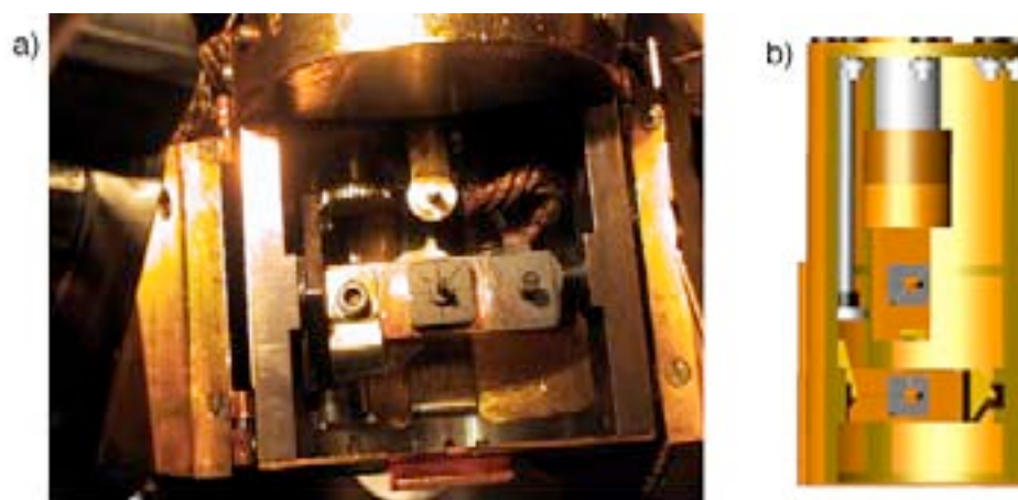
Figure 2.17: (a) Low-temperature sample manipulator at BL 5-4 with cleaved sample. (b) CAD drawing of the HeLM low-temperature manipulator.
