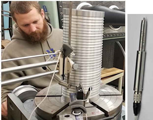
Figure 6: a) Measurement of alignment in a 30-washer stack; b) Microsense model 6530-LR-06 capacitive probe. surface finish was <1 \mu\text{m} . Each spacer washer is precision-ground on both faces to a thickness uniformity of <1 \mu\text{m} .
