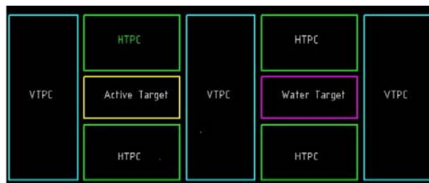
Figure 2. Schematic view of the new design under study for the ND280 upgrade. VTPC (HTPC) stands for vertical (horizontal) TPC.
