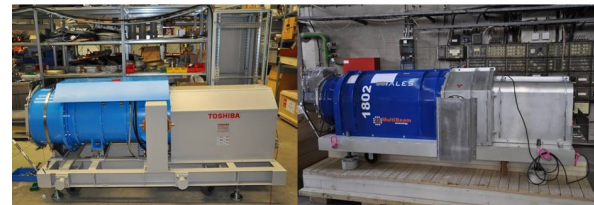
Figure 5: Multi beam klystrons for the E-XFEL.
