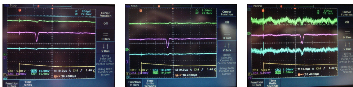
Figure 8. First LT signals seen at the AMT. Left to right correspond to heights of 2.0, 4.9 and 8.5 km a.g.l. Each panel shows 3 signal traces, averaged over 128 laser pulses, by PMTs in the same row. As the path length gets longer, signals shift further in time relative to the external trigger pulse (bottom trace).
