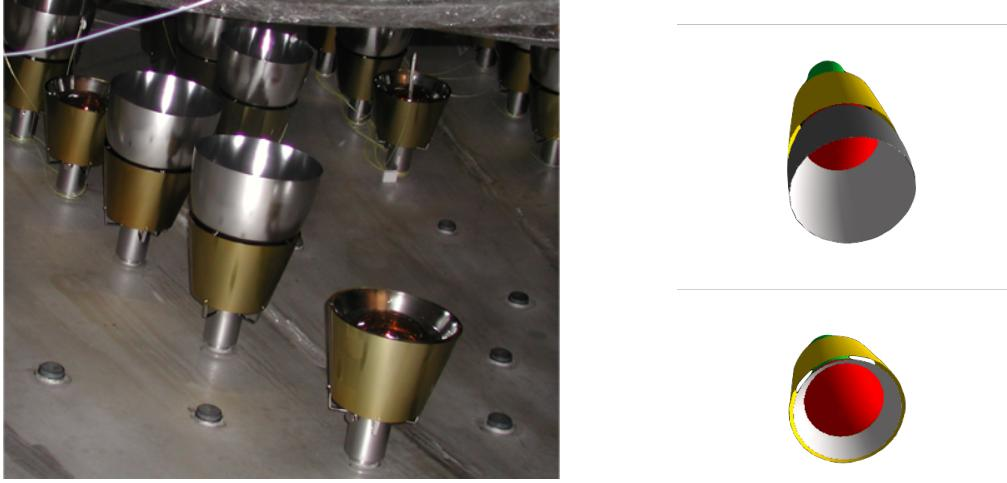
**Fig. 5.4:** *Left Panel:* Borexino ID PMTs mounted on the SSS. *Right Panel:* MC schematization of the PMTs with (top) and without (bottom) concentrators.
