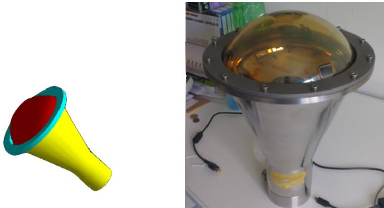
**Fig. 5.2:** Comparison between the schematization of the OD PMTs in the simulation and the actual objects.
