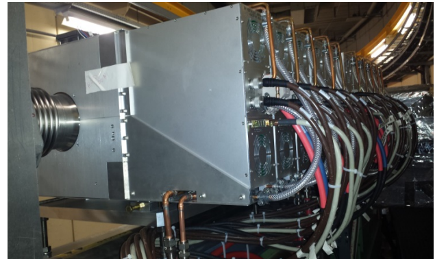
Figure 1: 10-cell prototype MA cavity in PSB Ring 4.
