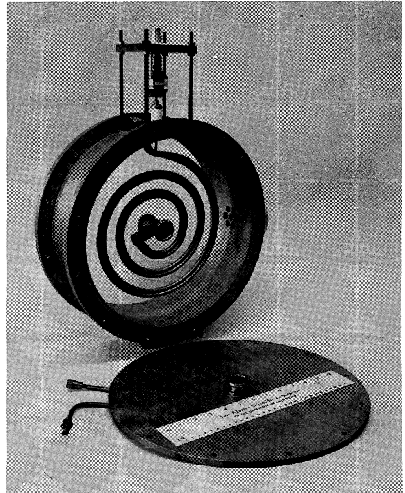
FIGURE 6 Photograph of resonator B with the end plates removed. A 120 pF vacuum coupling capacitor is shown at the top of the figure. This resonator was operated at 2.6 MV/m without the use of feedback control circuits.
