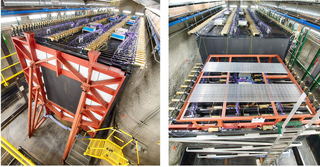
Figure 2.10: Top view images of the ND. The left picture shows the front of the ND showing the full active region, the right picture shows the back of the detector showing the muon catcher.
