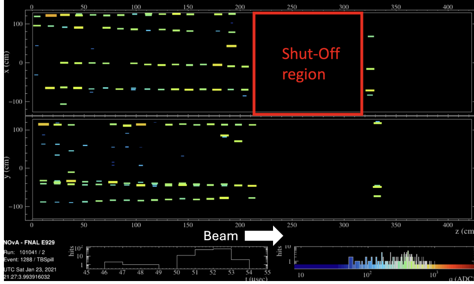
Figure 6.7: NOvA Test Beam Event Display showing the top and side view of the detector, the shut-offs can be seen as blank regions in the detector. The tertiary beam direction is indicated by the arrow.
