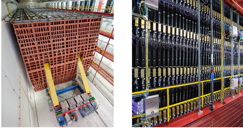
Figure 2.11: Far Detector photographs. The left picture shows the front of the FD, the right picture shows a section of the detector depicting the NOvA planes (in black), the FEBs (in gold) and the DCMs (silver).
