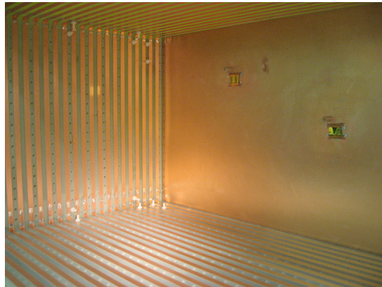
Figure 5.13: A look inside the TPC. The solid copper sheet is the cathode plane and the copper strips lining the TPC are the field cage rings. The TPC frame (i.e. what the copper is attached to) is composed of G10.
