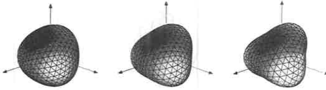
Figure 4: The tetrahedral surfaces for three different values of the deformation parameters \alpha_{32} = 0.1, 0.2 and 0.3 , respectively.
