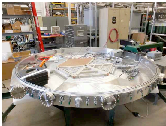
Figure 3: The 80 K beam chamber that will be filled with low pressure He gas. (The chamber cover is not shown.)
