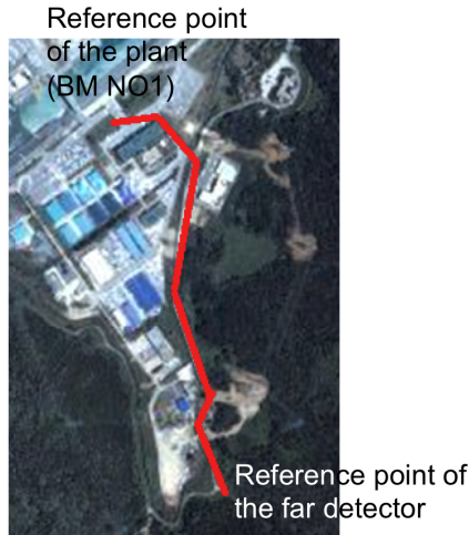
Figure F.5: Satellite map of survey route for Z position of detector center. Red line is survey route by the Soobong construction from level reference point (BM NO1) of the plant to reference point of the detector.
