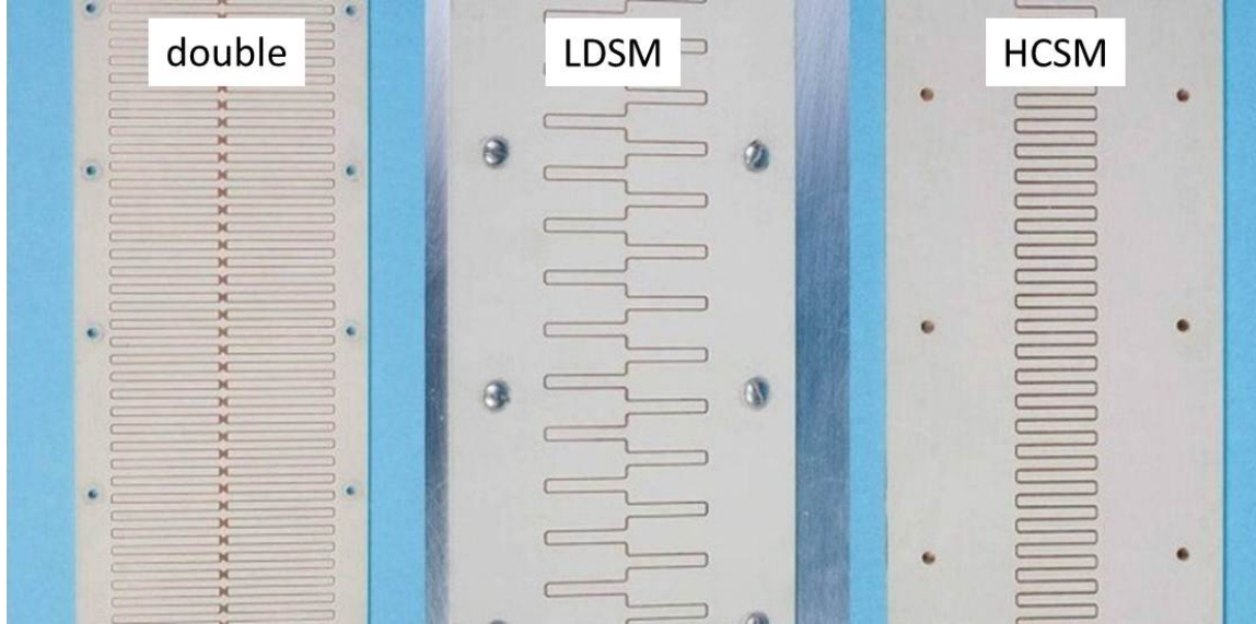
Figure 4. Three prototype microstrip deflecting structures. From left to right: the 50\ \Omega double meander, the 100\ \Omega low dispersion single meander (LDSM) and the 100\ \Omega high coverage factor single meander (HCSM).
