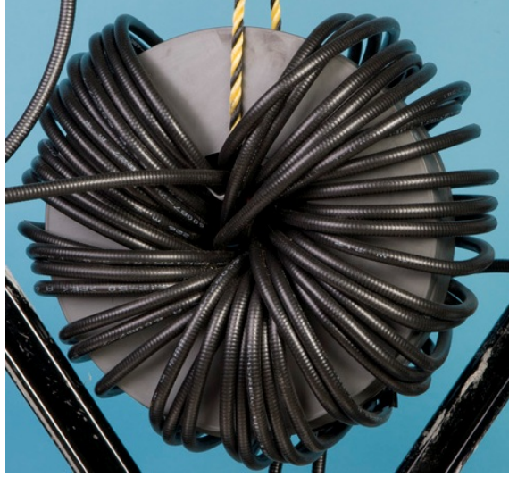
Figure 11. One combiner with \frac{3}{8} " Heliax superflexible cable and five 1" thick MN60 ferrite cores.
