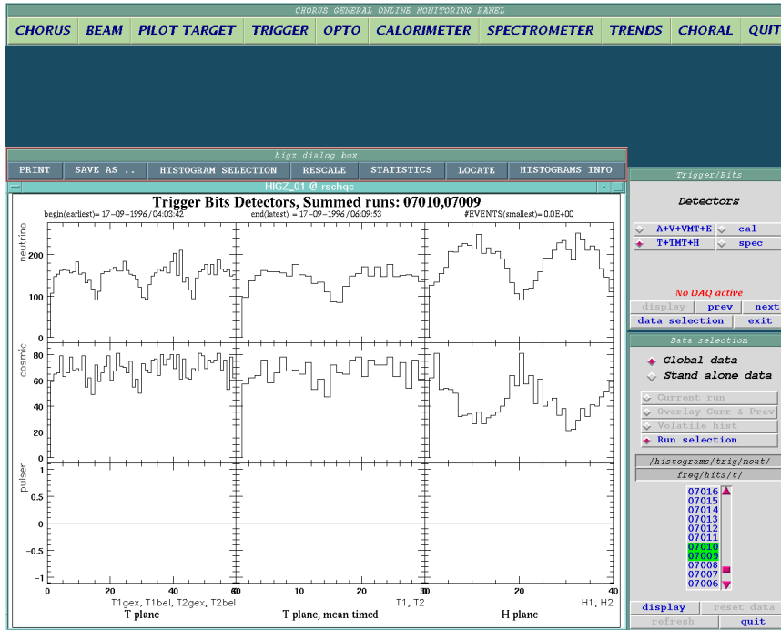
Figure 2.14: The online monitoring histogram viewer. As an example the hit distributions of the trigger planes T (singles and mean-timed) and H are displayed for neutrino events and cosmic events and for trigger calibration events (pulser) for the runs 7009 and 7010.
