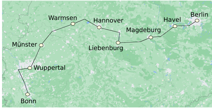
Figure 5.8: Map of Germany overlaid with a depiction of the fiber path connecting the German cities of Bonn and Berlin that we investigated. The white circles represent end nodes, in Bonn and Berlin, and repeater nodes elsewhere. This placement corresponds to the best found by our optimization method, in the sense that it allowed for minimization of hardware requirements for a target secret-key rate of 10 Hz.
